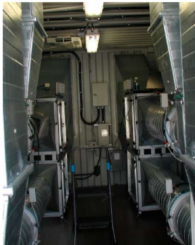
CamField Lab interior - four separate test ducts
